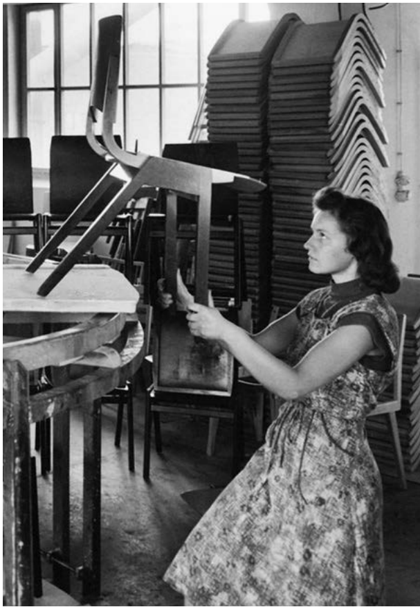
The 21A stackable chair by architect, urban planner and designer Roland Rainer was produced between 1958 and 1966. The A-shaped frame made of solid beech made it possible to stack large numbers of chairs on top of one another. → Aula , page 67
