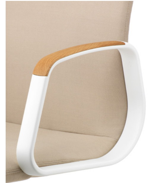
Armrest made of die-cast aluminum, coated white with a textured matte finish with an embedded armrest pad made of solid oak
